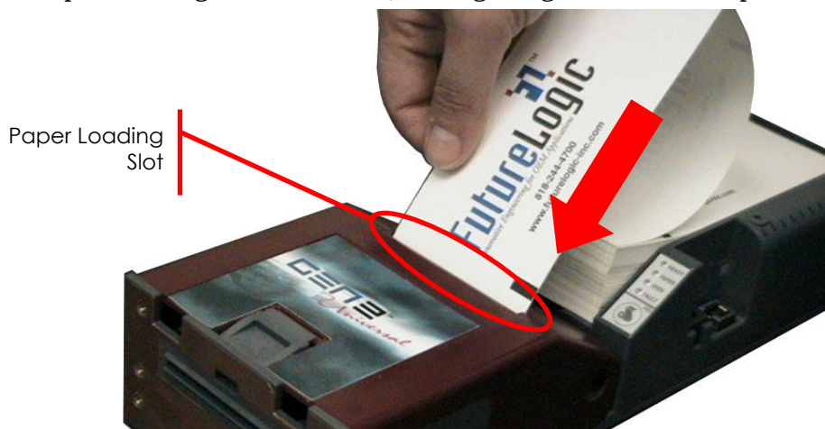
Figure 3-3 Feed Paper into Paper Loading Slot
