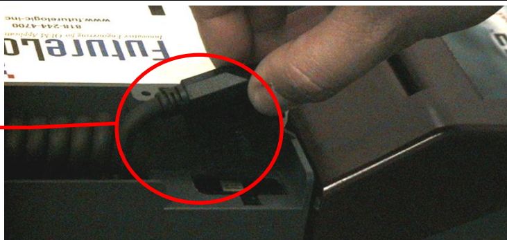
Figure 4-2 Disconnect the Coiled Cable Connector
