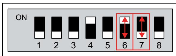
Figure 6-70 DIP SW1 #6 and #7 ON
