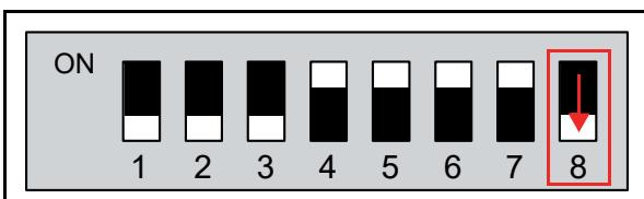
**Figure 6-79** LED Test DIP SW1 #8 OFF
